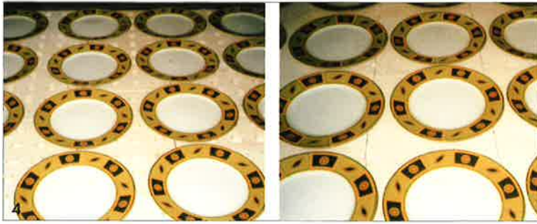
Fig. 4 Kiln car with decoration firing kiln feed: left side new system, right side old system (repairs with mortar at the edges of the insulating bricks)
