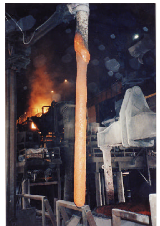
Figure 13. A refractory-covered lance used for injecting desulphurizing agents and gases into molten iron and steel to improve metal quality. The refractory experiences both thermal shock and corrosion by slags as evidenced by the neck down in the zone
