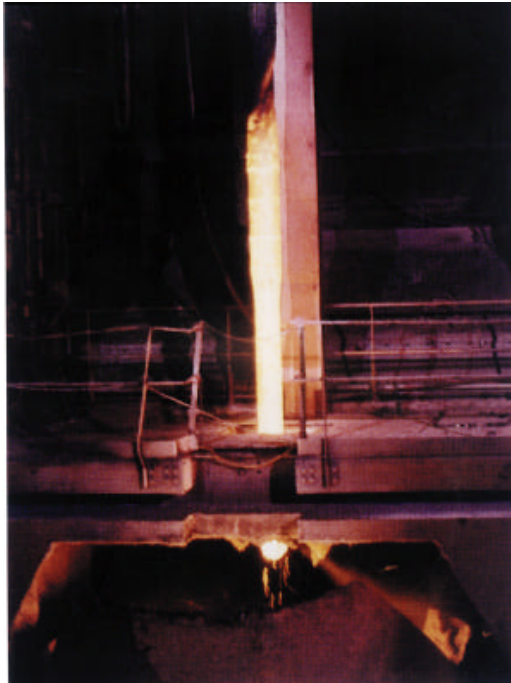
Figure 14. Another lance just as it is removed from the ladle. The necked-down region did not occur on this lance. Alphabond along with magnesium aluminate spinel in the castable will improve slag and thermal shock resistance.
