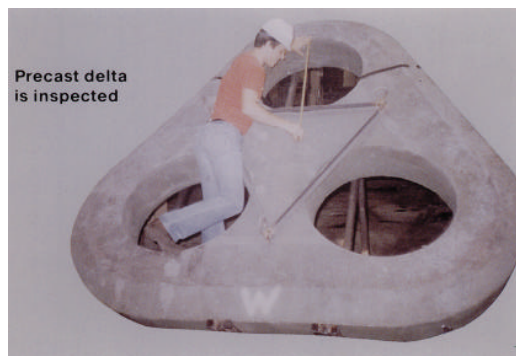
Figure 15. A precast electric furnace delta section 20 inches thick. Significant improvements in life have been observed with castables which contain Alphabond; however, these sections must be fired carefully to avoid explosive spalling.
